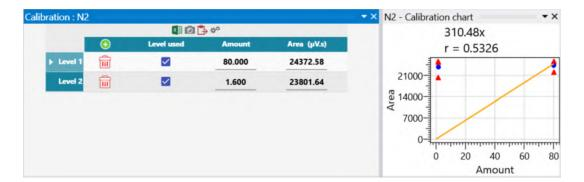
From this moment, if an analysis is started with the "Analysis" method, the chromatogram obtained will be automatically processed with the integration method and the identification table previously developed and the result in concentration will be linked to the calibration previously performed.
