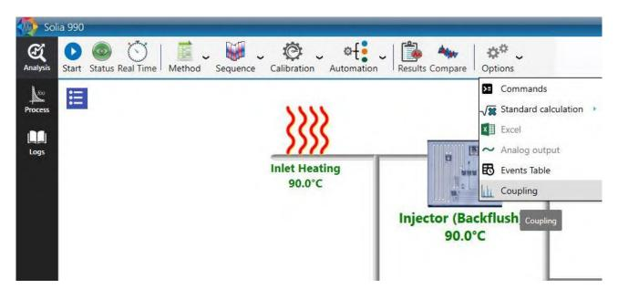
A window will then open. Select "Solia" and then the name of the MS instrument created in the Agilent GCMS configurator, as below:
