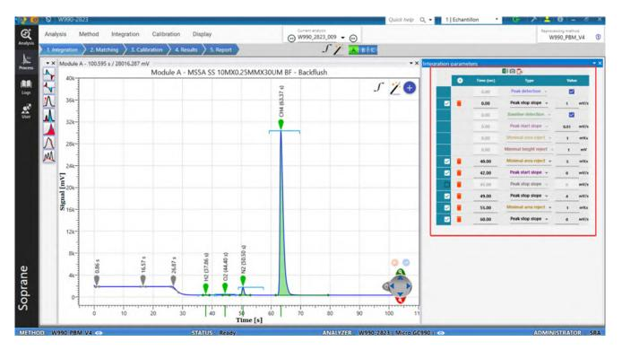
The "Integration Parameters" are used to define how to integrate the peaks on the chromatogram. In the "Integration Parameters" table, a row corresponds to an integration parameter. For each line, it is necessary to define the "Time" from which the parameter must be applied until the end of the chromatogram or the definition of another similar parameter, the "Type" of integration parameter to be applied and its "Value".
