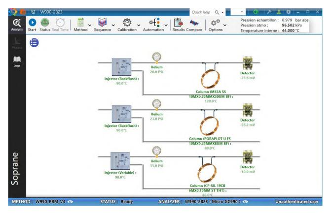
If an element has not reached its set point, it means that it is not ready. The text is in Orange.
