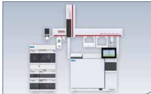
Off-line preparative techniques (LC, LLE) are replaced with an automated separation of the fractions of interest via HPLC. This analytical approach also allows to eliminate the saponification step.
