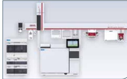
Off-line preparative techniques (LC, TLC, LLE) are replaced with an automated separation of the fractions of interest via HPLC.
