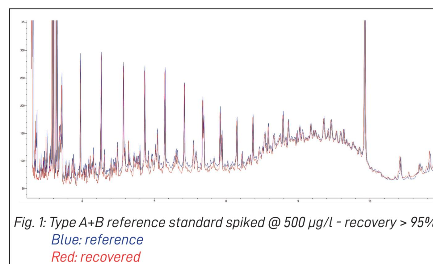
Fig. 1: Type A+B reference standard spiked @ 500 µg/l - recovery > 95%
